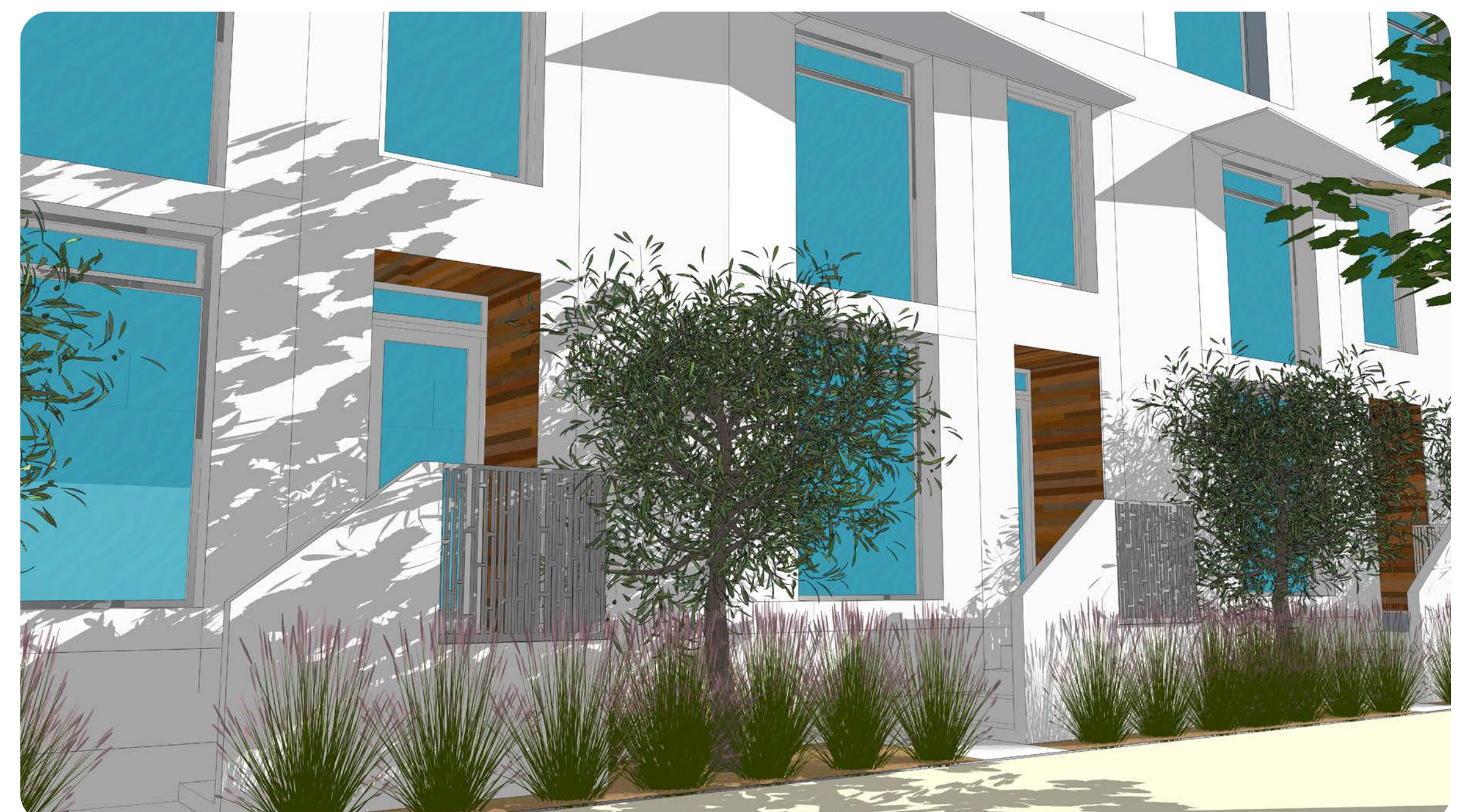
Ground floor entries to individual units shall be raised from the sidewalk and setback with a landscaped strip.
