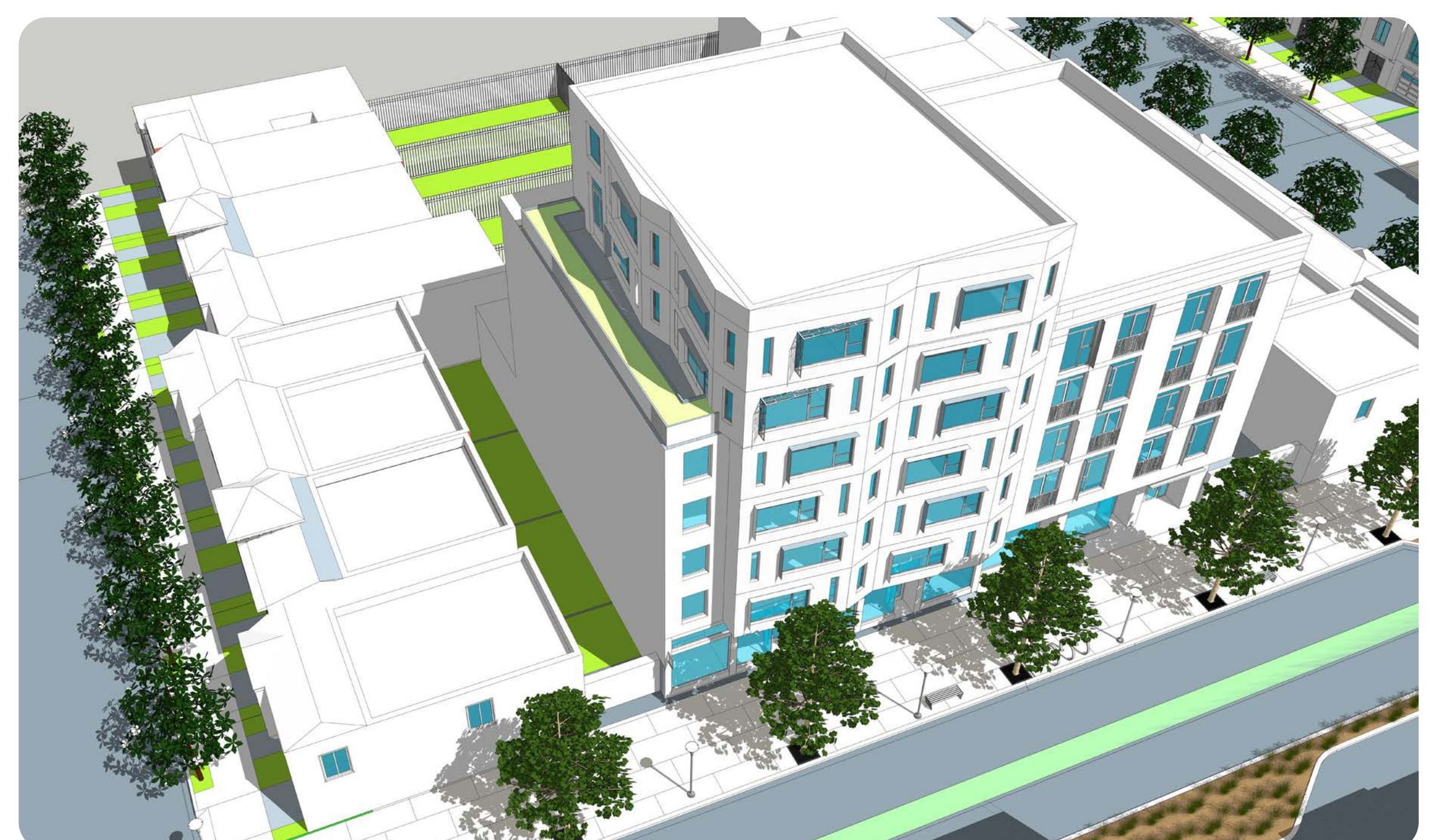
When the side of new housing abuts an existing rear yard volume must step back 10' at 55' height.
