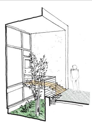
The front setback may be adapted to provide light and air to sub-grade habitable space that is part of a 2-story unit.
