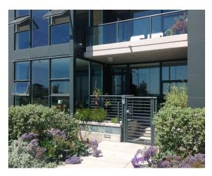
Use a covered entryway combined with a modest setback to create an inviting entryway and usable terrace. Although only slightly elevated, most of the setback is used for landscaping to screen the terrace from the sidewalk.
