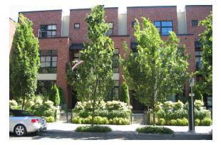
Provide raised and generous setbacks (approximately 8 feet), with significant landscaping to provide greater privacy; modulate the building and detailing to clearly identify individual units; recess the entries to provide protection. Layer the landscaping to further screen the ground floor units.
