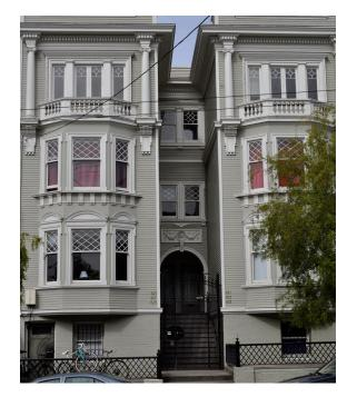
Use entrance systems, such as this exterior stair, to vertically modulate the building and provide variation in the street wall.
