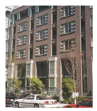
Use entries to modulate the building horizontally by defining a base, and vertically by establishing a regular interval along the facade. Using high inset entries (at least two stories) may allow a lesser setback of the entire building.
