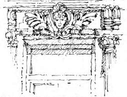
Cornices are an example of an architectural feature that should be rstored, retained, or recreted. Contemporary materials, such as Glass Fiber Reinforced Concrete (GFRC) or Fiber Reinforced Polyester (FRP), may be employed as a substitute for terra cotta, cast stone, or pressed metal. Ghosting, scaring, and other visual evidence may help explain alterations to building features and openings over time.
